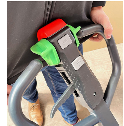
Secondary emergency stop at the top of the control handle
