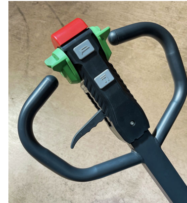
Fork lifting, lowering and drive controls
