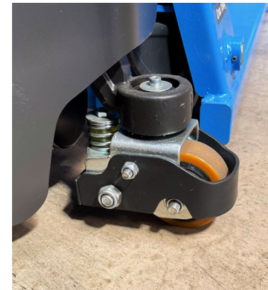
Fully enclosed drive wheel and protected rear castors
