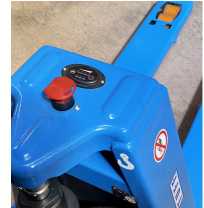
Emergency stop, on/off, battery and fault code indicator
